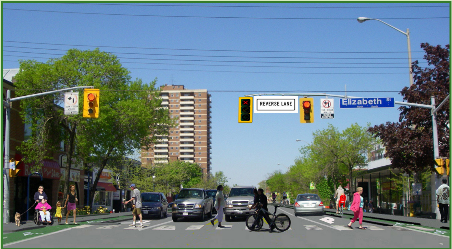
Rush-hour reversible centre lane with on street parking, moving east in the morning and west in the evening. Also present are widened sidewalks, physically separated bikelanes, and bus stops.
