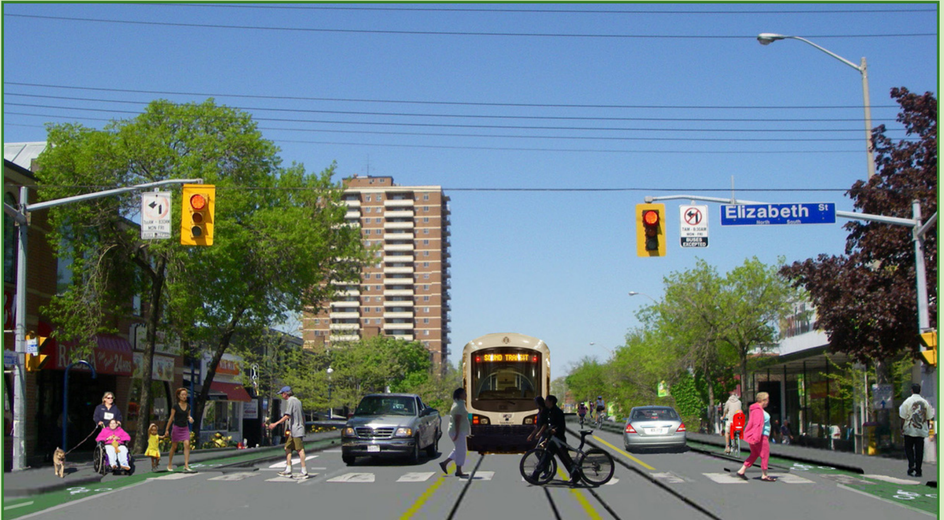
Street car expansion with two rails along Lakeshore road with parking on north side, widened sidewalks, bus stops, and physically separated bike lanes.
